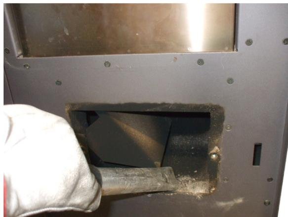
**Fig. 31 - Fume chamber cleaning**
