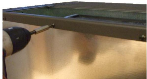
Fig. 16 - Backward screws removal
