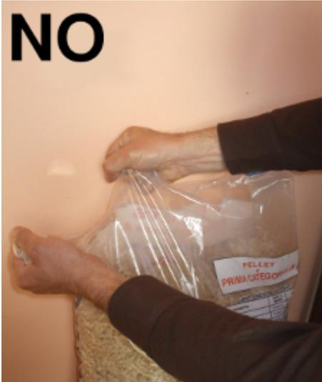
Fig. 23 - Wrong opening of the pellets bag
