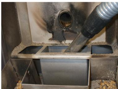
Fig. 27 - Burning pot box cleaning
